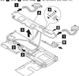
Do 4 and 5 after step 3 to remove the rear IR.
